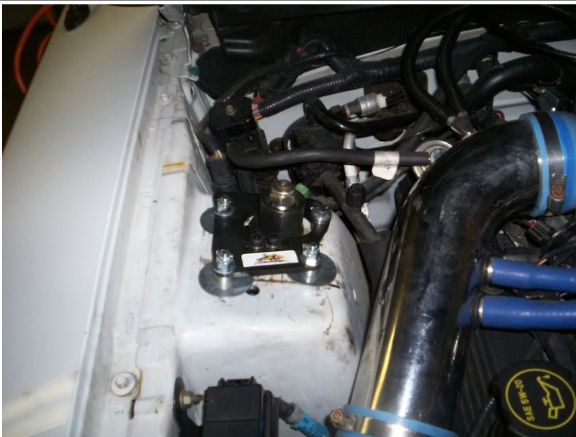
Granatelli coil overs installed. Some tight tolerances, but using your head and COMMON SENSE will get you through this.
