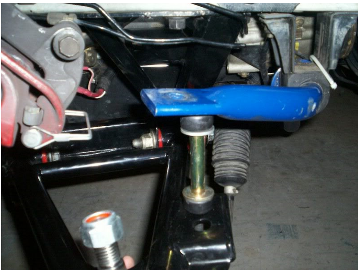
Adapter to move swaybar foward one inch using OE hardware
