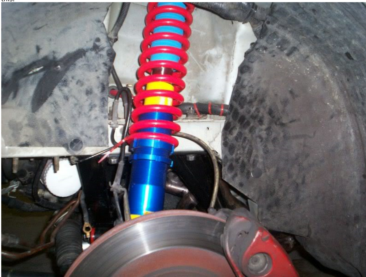
Granatelli coil overs installed. Some tight tolerances, but using your head and COMMON SENSE will get you through this.
